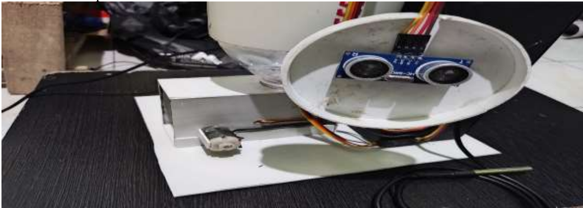
Figure 16. Installation of Temperature and Ultrasonic Sensors
