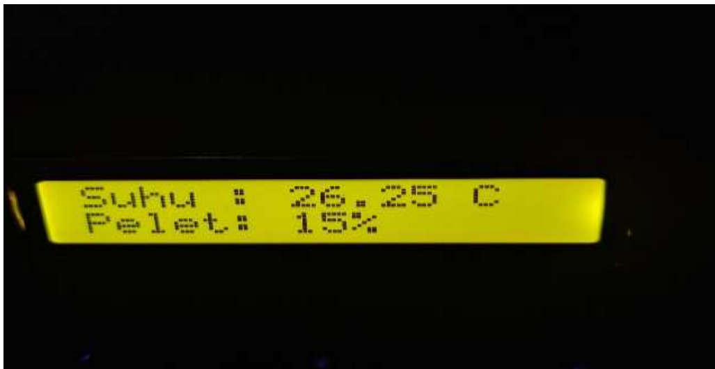
Figure 9. Pellet level display on LCD
